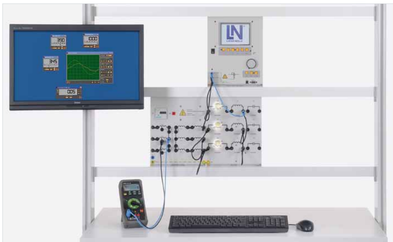
Experiment example: "Transformer trainer ENT 5"
