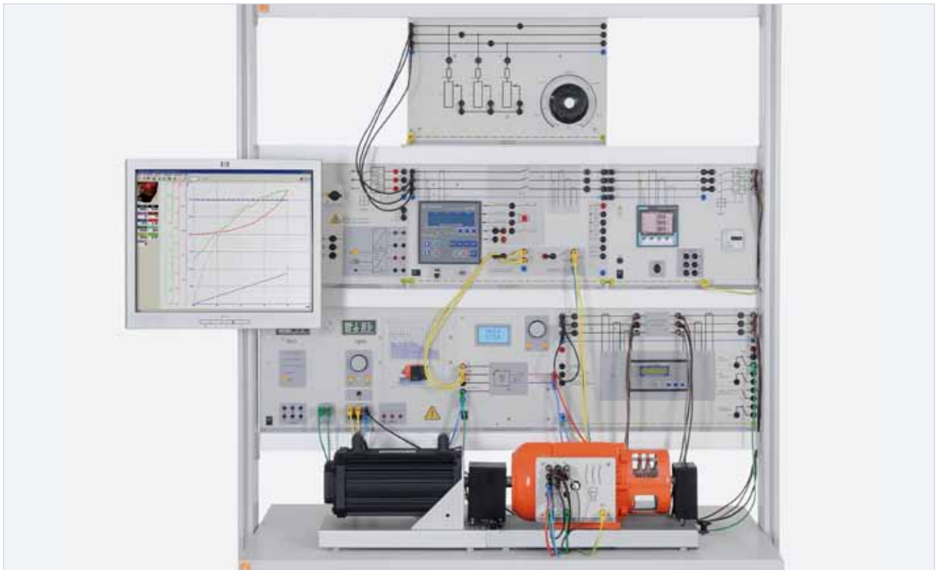
"Generator differential protection" EGP 2
