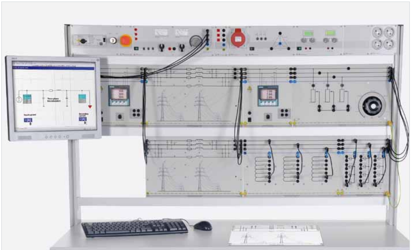
Sample experiment "Investigations on parallel lines" EUL 2
