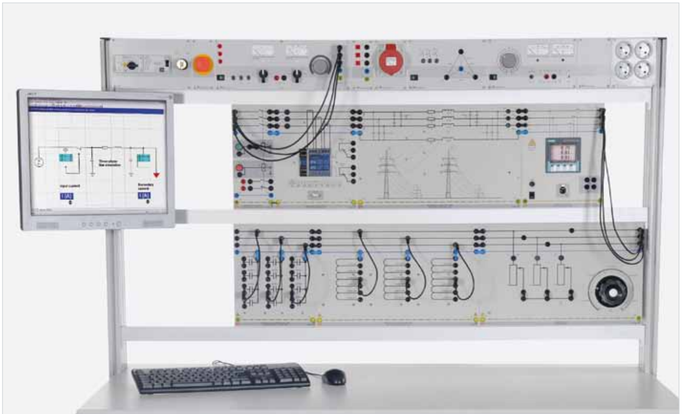
Sample experiment "Overcurrent time protection for lines" ELP 1
