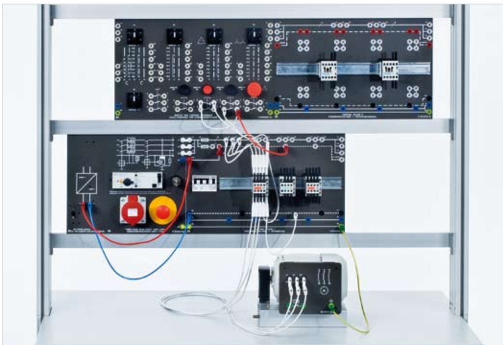
Experiment example "Contactor circuits in a three-phase circuit EST 2"
