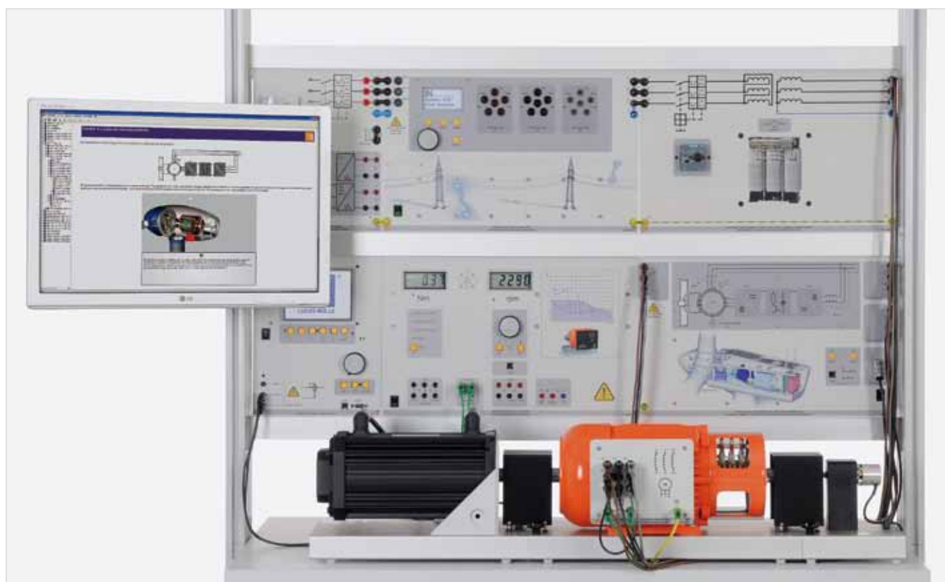
Sample experiment "Wind power plant" EWG 1
