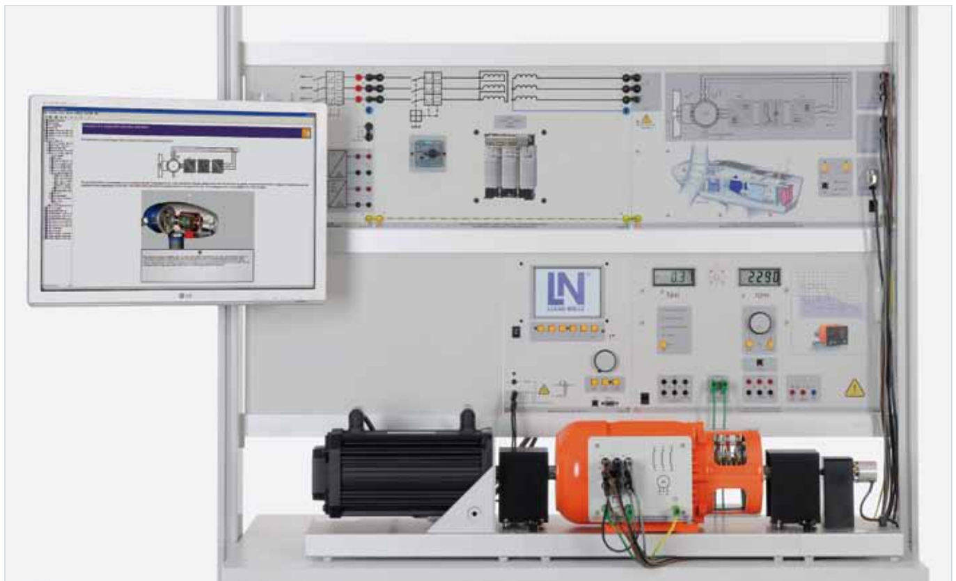
Sample experiment "Small wind power plant" EWG 2
