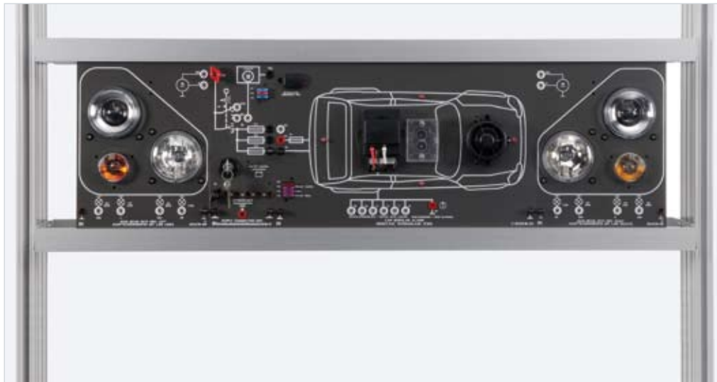
Sample experiment: "Alarm system and immobilizer"
