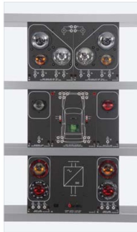
Experiment: "Vehicle lighting control via CAN bus" with a SO3216-2Z interface and additional components
