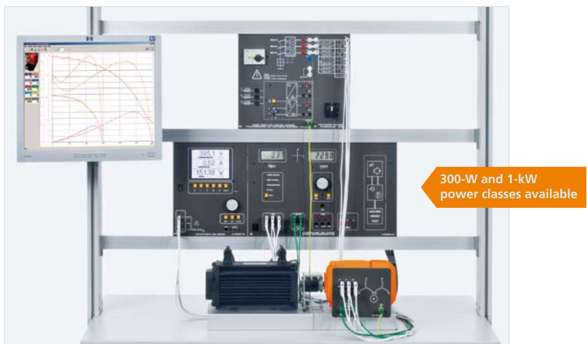
Experiment example: "Three-phase pole-switchable motor with two separate windings EEM 4.3"
