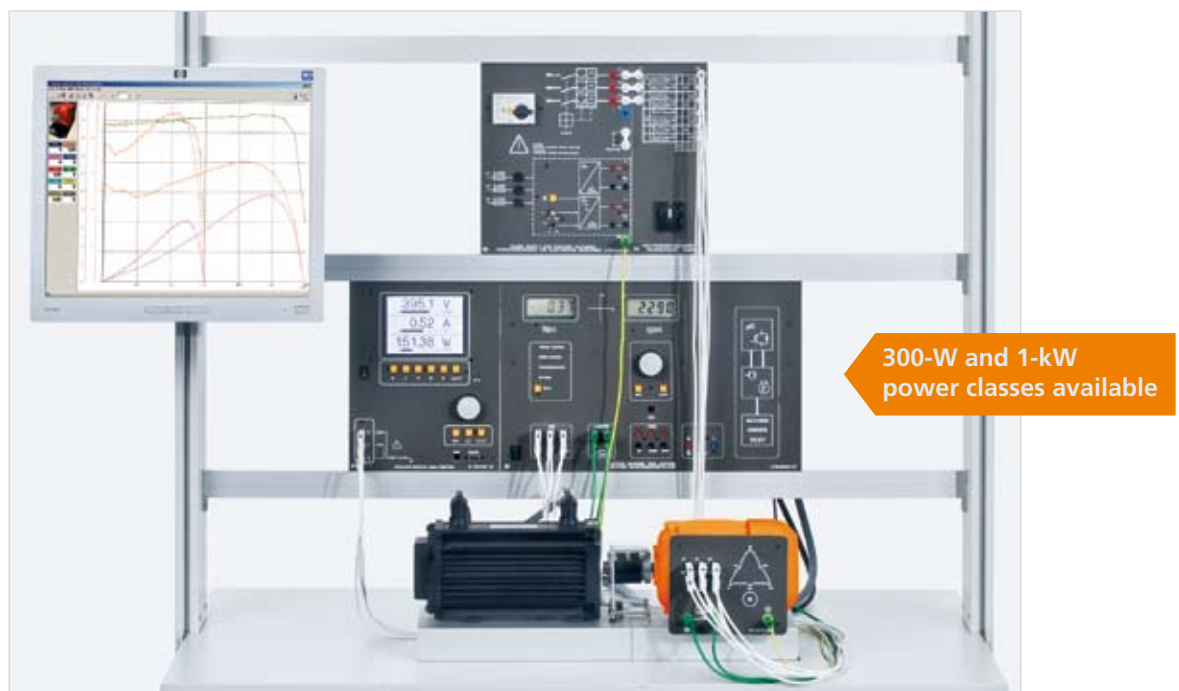
Experiment example: "three-phase pole-switchable motor according to Dahlander EEM 4.2"
