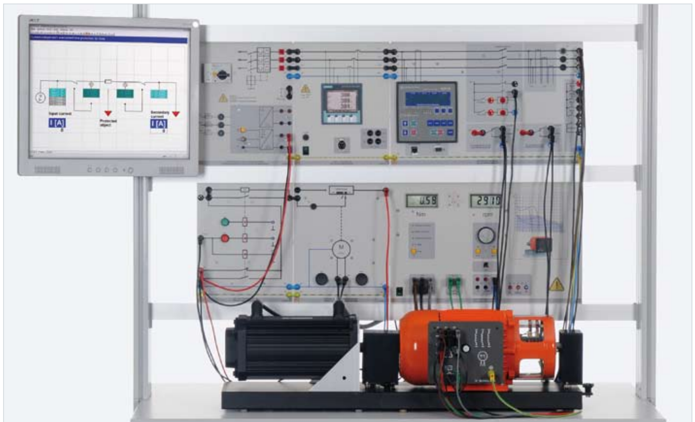
Sample experiment "Generator protection" EGP 1
