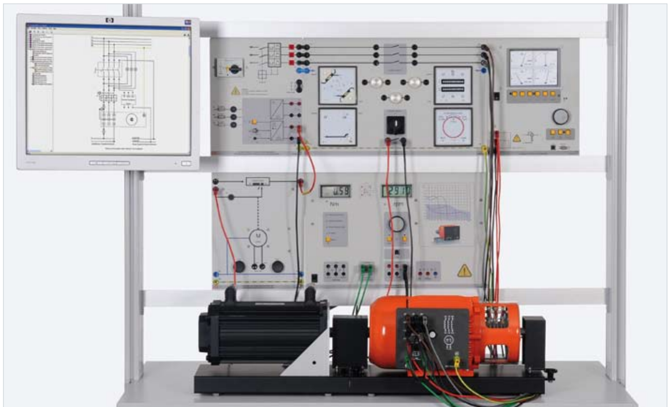
Sample experiment "Manually operated synchronising circuits" EUG 1
