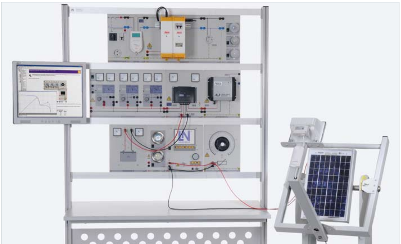
Sample experiment "Advanced photovoltaics" EPH 2
