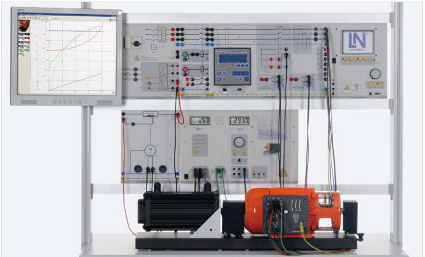
Sample experiment "Automatic synchronising circuits" EUG 2
