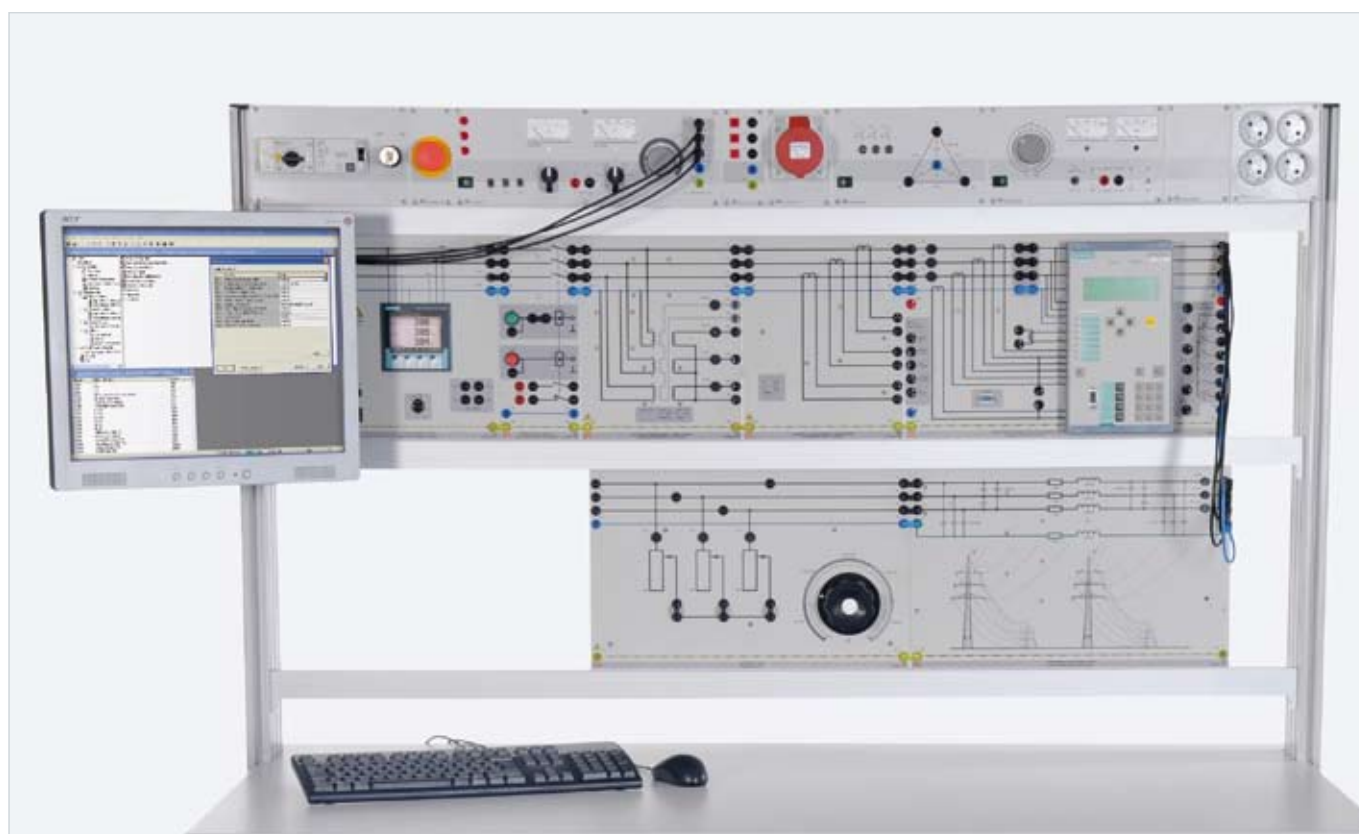
Sample experiment "High-speed distance protection" ELP 7
