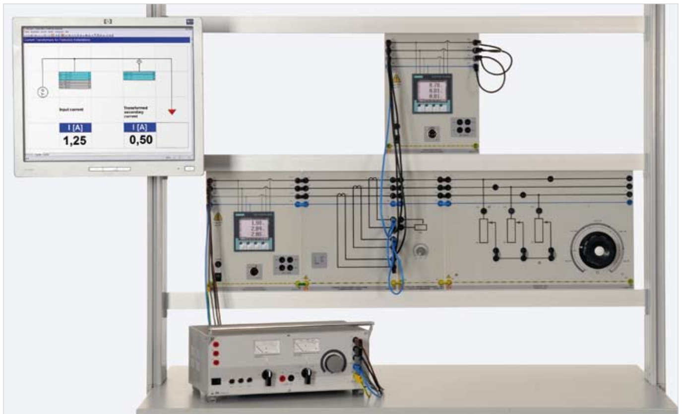
Sample experiment "Current transformer" EUB 1
