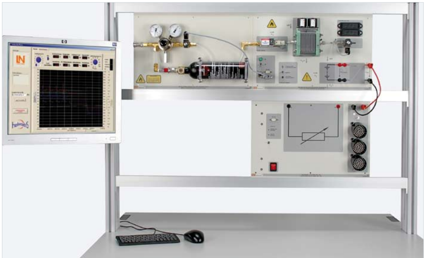
Sample experiment "50-VA fuel cell stack with loads" EHY 1
