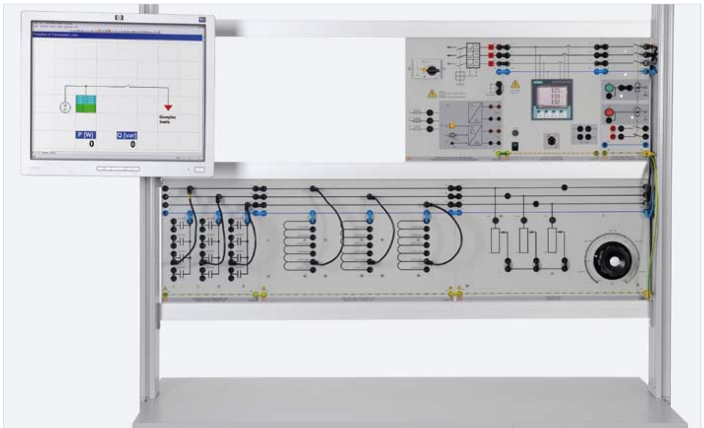
Sample experiment "Measuring the power consumption of complex loads" EUC 1
