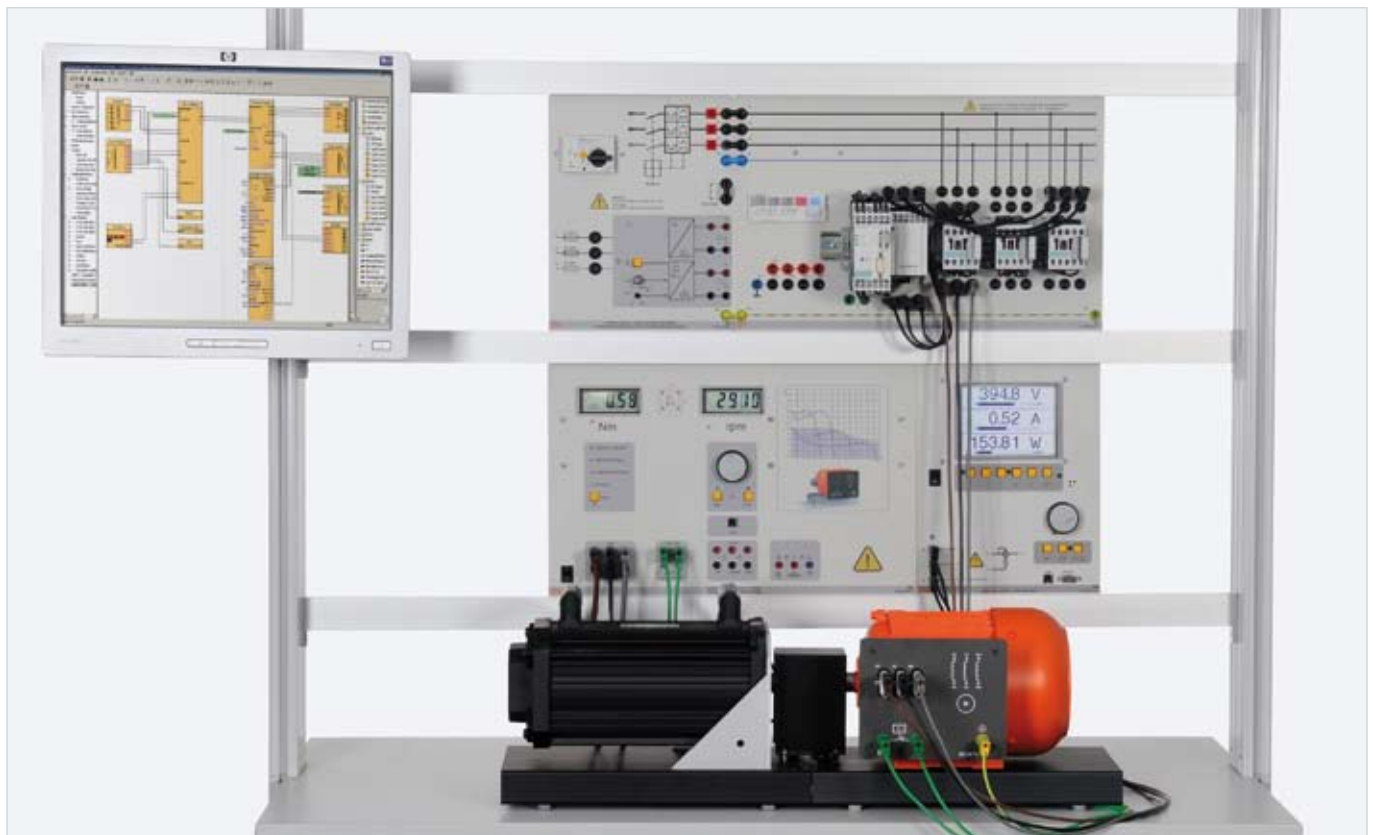
Sample experiment "Motor management relay" EDT 51
