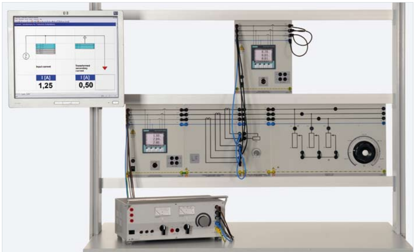
Sample experiment "Current transformer" EUB 1
