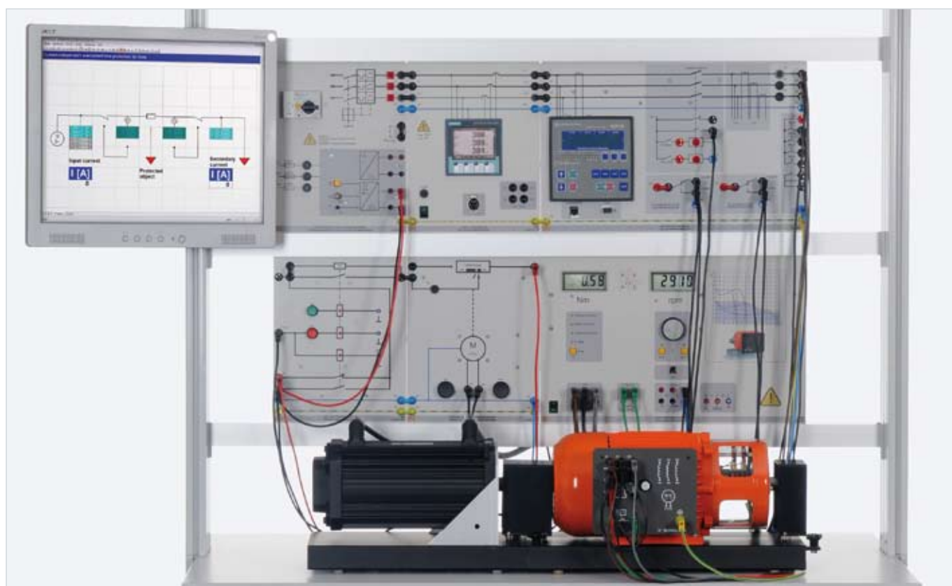
Sample experiment "Generator protection" EGP 1
