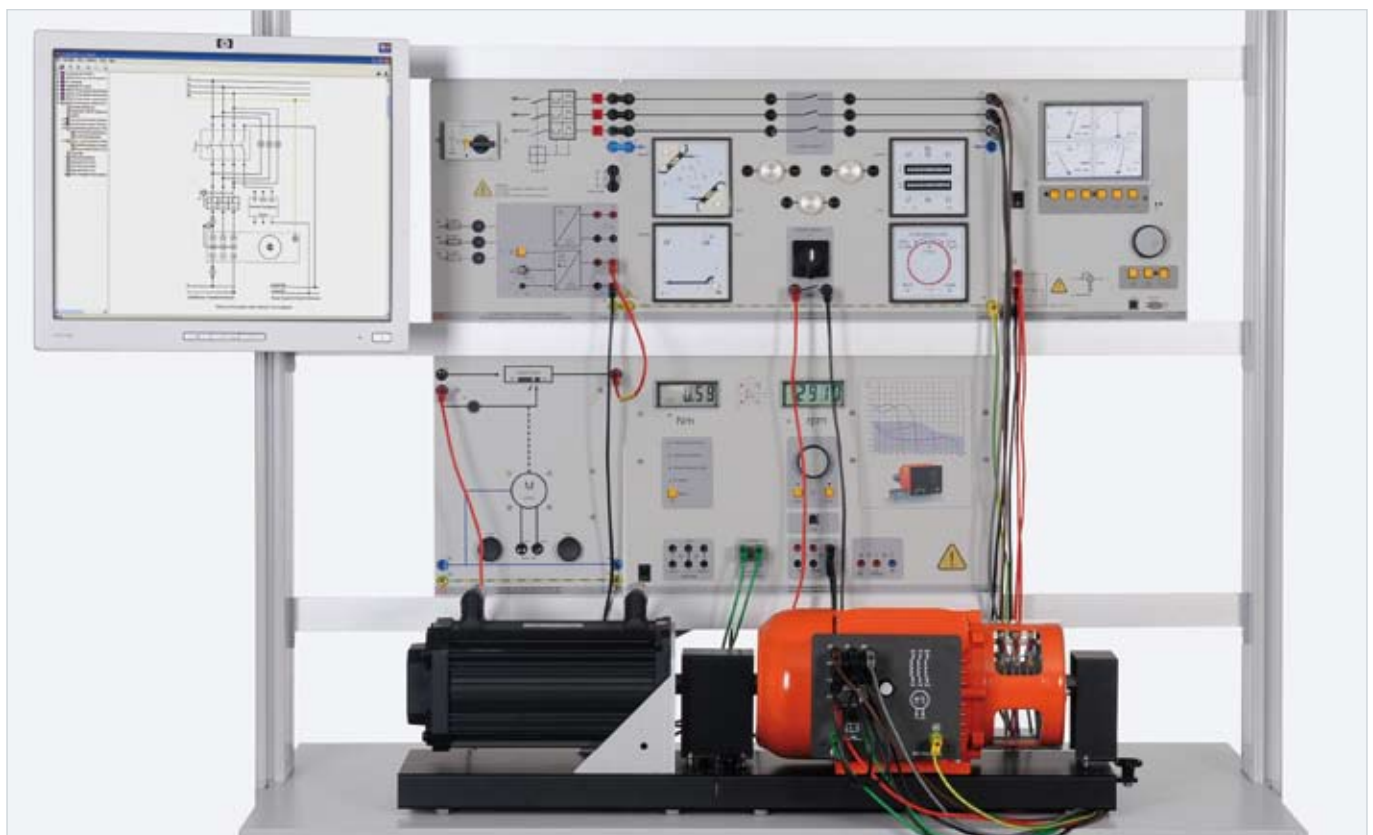
Sample experiment "Manually operated synchronising circuits" EUG 1
