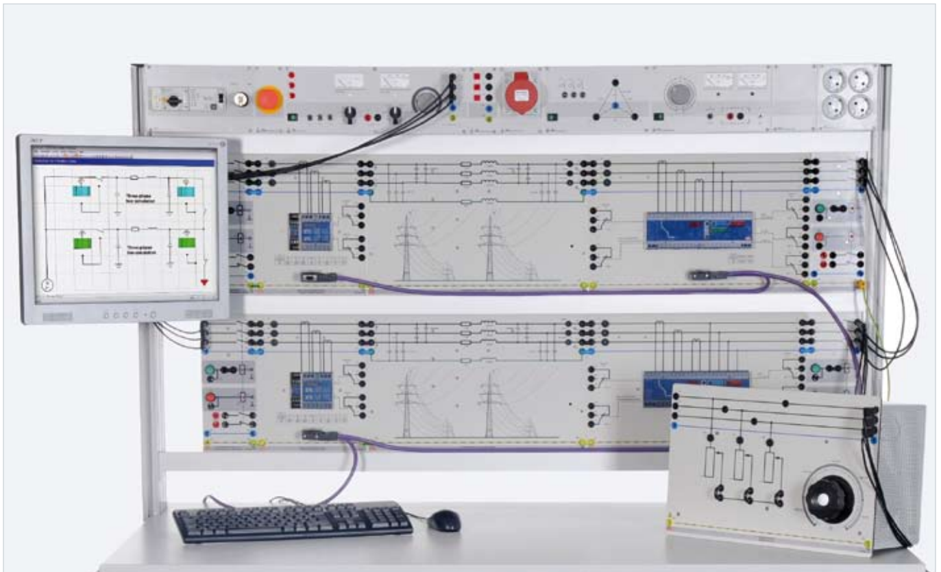
Sample experiment "Protection of parallel lines" ELP 6
