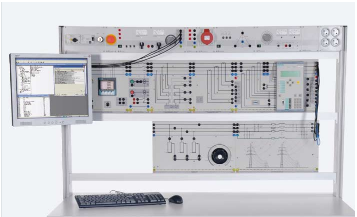
Sample experiment "High-speed distance protection" ELP 7
