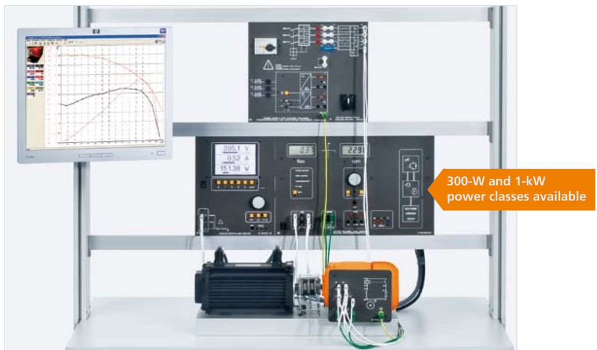
Experiment example: "Single phase motor with bifilar starter winding EEM 3.3"
