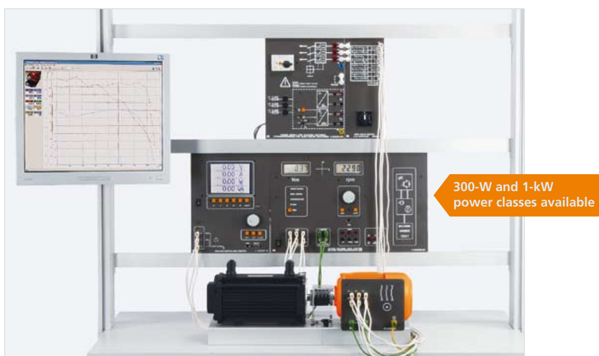
Experiment example: "Three-phase motor with squirrel-cage rotor EEM 4.1"
