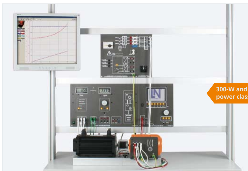
Experiment example: "Three-phase reluctance machine EEM 5.3"
