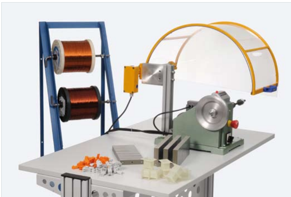
Experiment example: "Winding transformer coils EMW 10"
